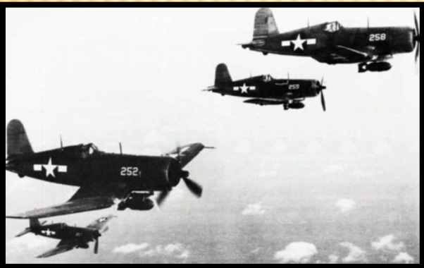
*Image info: Four U.S. Marine Corps Vought F4U-1 fighters armed with bombs in late 1943 or early 1944. (U.S. Government photo/released).
